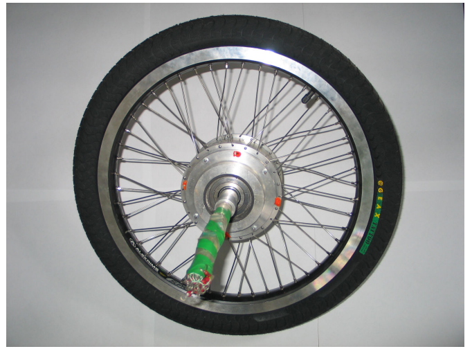
Fig. 1. Prototype external-rotor motor fitted within a wheel- hub
