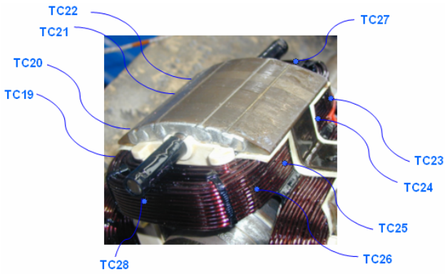
Figure 3: Location of rotor thermocouples.
