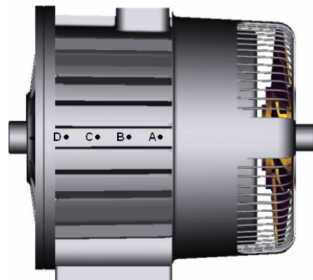
Figure 5: Air flow measuring points of the UC22B frame.
