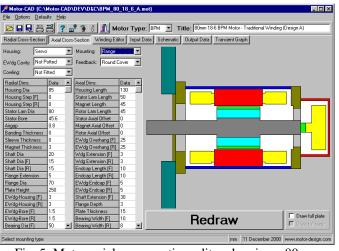
Fig. 5: Motor axial cross-section editor showing a 80mm diameter traditionally wound motor design
