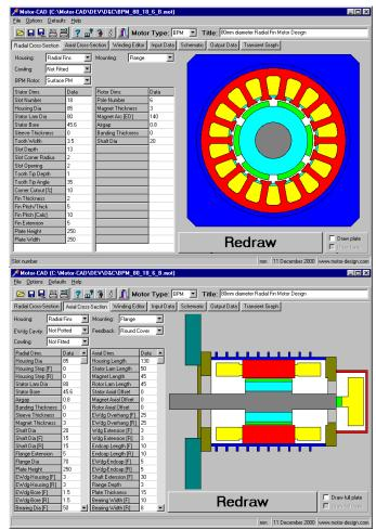
Fig 8: Motor with a radial fin design
