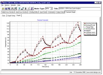
Fig. 11: Thermal transient for a small servo motor operating a duty cycle type load (load shown in Fig 12).
