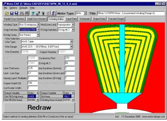
Fig. 7: Winding model showing the high slot-fills achievable in a precision wound non-overlapping winding
