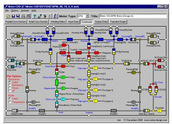
Fig. 1: Motor-CAD lumped circuit BPM thermal model
