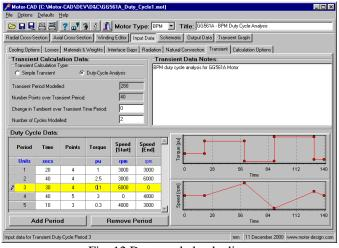
Fig. 12 Duty-cycle load editor
