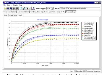
Fig. 10: Comparison of measured and calculated thermal transient for a small servo motor
