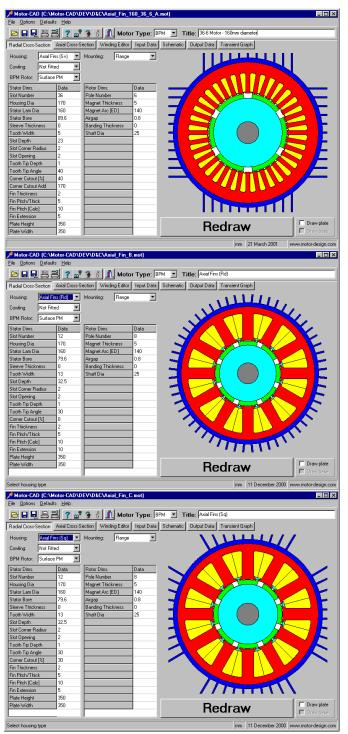
Fig 9 Examples of axial fin types available in Motor-CAD
