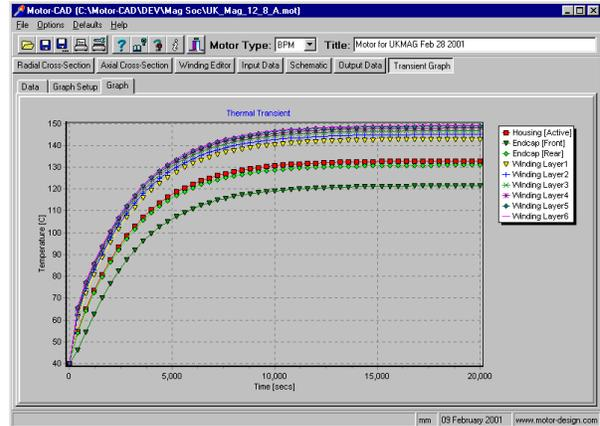
Fig 9: Motor-CAD - thermal transient with full-load
