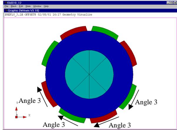
Fig 4: Offset angle used for half motor magnet group
