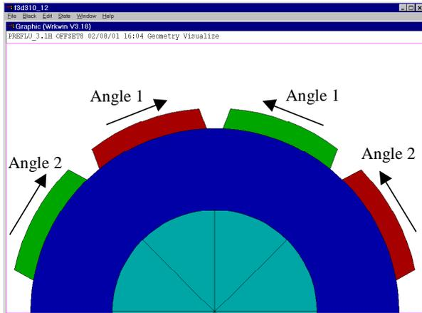
Fig 2: Offset angles used for half motor individual magnets
