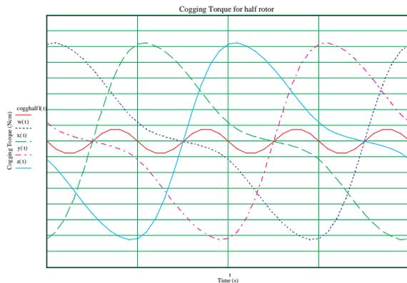
Fig 3: Cogging waveform for half motor with offset magnets
