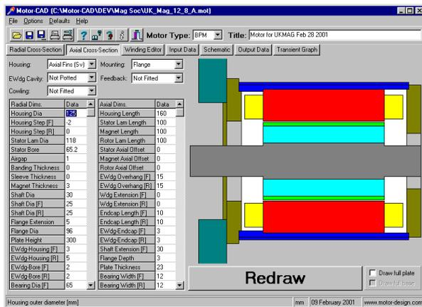
Fig 8: Motor-CAD - radial & axial screen cross-section
