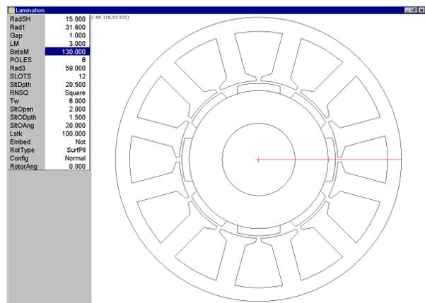
Fig 6: PC-BDC - radial cross section of 12-slot 8-pole motor
