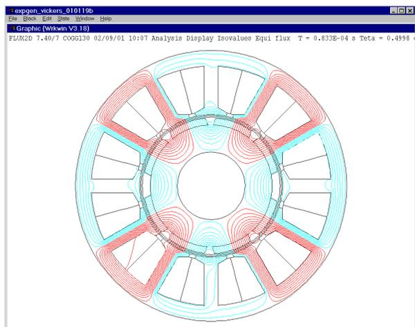
Fig 10: Flux-2d - offset magnet motor flux plot
