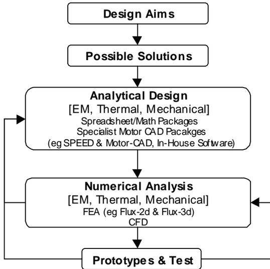
Fig 1: Flow diagram of design process used by authors
