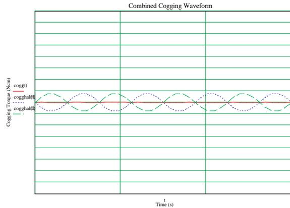
Fig 5: Cogging waveform for two half motors + total cogging
