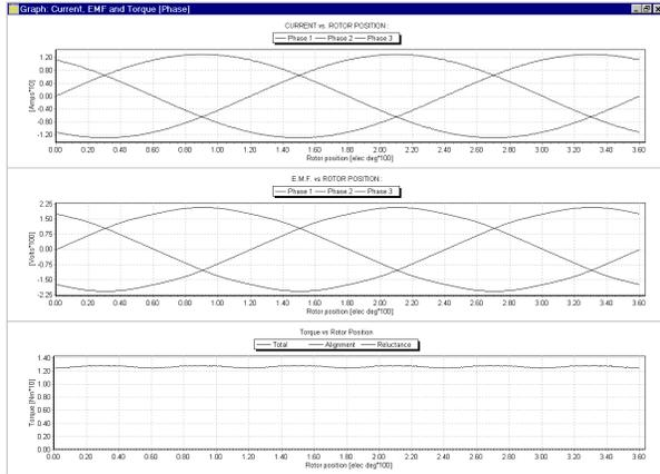
Fig 7: PC-BDC - prediction of rated current, emf & torque
