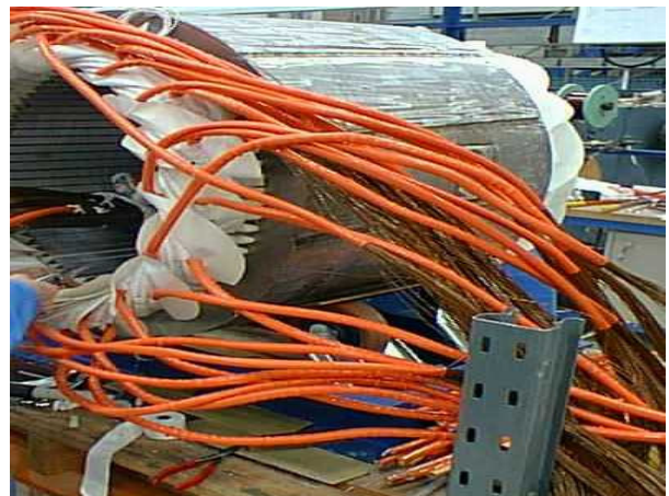
Fig.2. showing the stator pack and the winding
