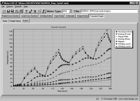
Fig. 13: Thermal transient for a small servo motor operating a duty cycle type load (load shown in Fig 14).
