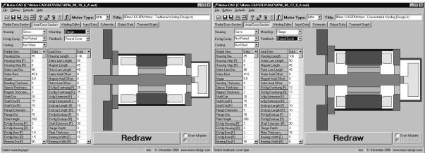
Fig. 3: Axial cross-section editor showing 80mm diameter traditional & concentrated winding motor designs
