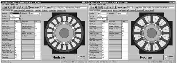
Fig. 2: Radial cross-section editor showing 80mm diameter traditional & concentrated winding motor designs
