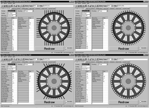
Fig 9: Examples of axial fin types available in Motor-CAD
