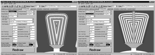
Fig. 6: Winding thermal model showing copper/insulation layers used in 80mm diameter traditional & concentrated winding motor designs
