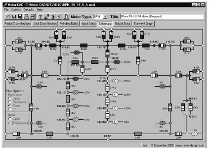
Fig. 1: Motor-CAD lumped circuit model showing resistance/node labels and power flow/nodal temperatures
