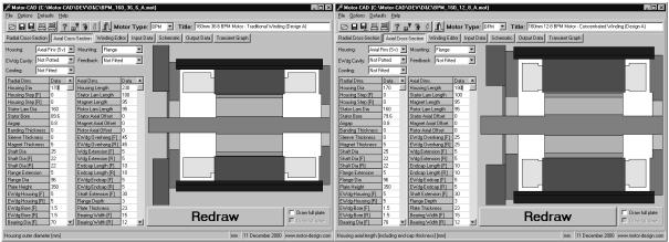
Fig. 5: Axial cross-section of 160mm diameter traditional & concentrated winding motor designs
