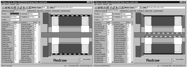
Fig 11: Example of liquid cooling arrangements available in Motor-CAD (housing & shaft water jackets)
