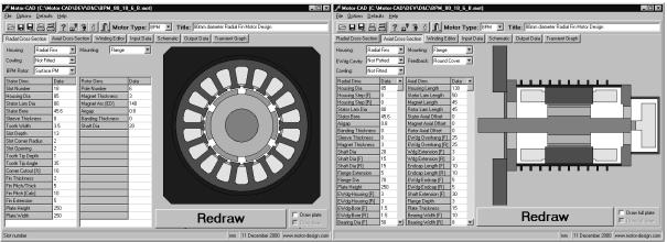
Fig 8: Motor with a radial fin design
