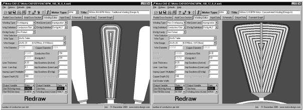
Fig. 7: Winding thermal model showing copper/insulation layers used in 160mm diameter traditional & concentrated winding motor designs
