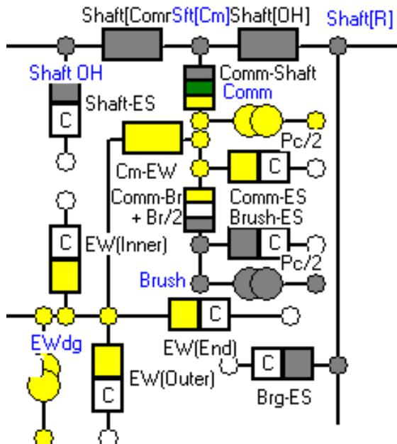
Fig. 9: Thermal network for the commutator and brushes
