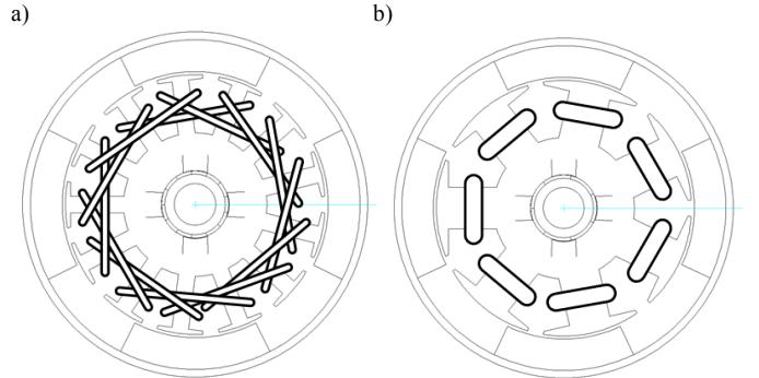
Fig. 6: Armature winding of calculated motors: a) Motors 1 and 2 (simplex wave winding); b) Motor 3 (single tooth winding)
