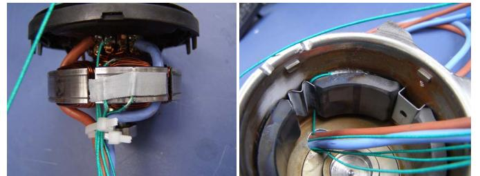
Fig. 5: Motor 3 rotor and stator with thermocouples attached
