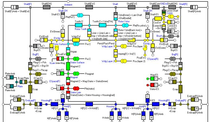
Fig. 8: Thermal network for the PMDC motor
