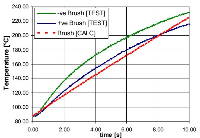
Fig. 11: Measured and calculated brush temperatures for the long Motor 2 (48A for 10 seconds).
